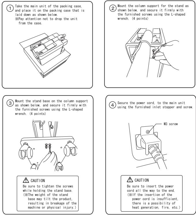
× Perform the following inspections at the end of the above-stated procedures. ·Check that all screws have been tightened. Be sure to check the screws at all nine points. •Check that the screws are fully tightened. Check for any loose screws at all nine points.
